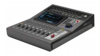
The LiveTouch20 is a 20 channels motorized faders digital mixer with large touch screen and USB ports. Full control is also available remotely via WIFI dongle provided to mix anywhere with your iPad. There are 12 Mic/Line inputs, 2 stereo inputs all routable via 4 mono busses, 4 stereo busses and master L/R. The 1024x600 touch screen makes navigation simple and intuitive for studio or live applications.
